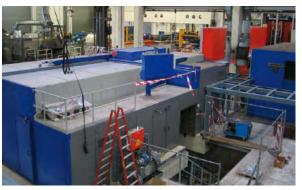
Operating weight Max. part diameter Bar diameter Strokes per minute Press force 950 – 7.500 g ca. 180 mm 45 – 90 mm 50 – 80 20.000 kN
